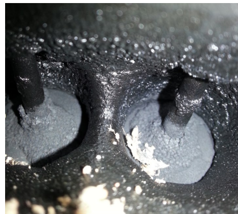
Carbon deposits on valves
